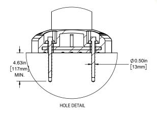
Customer Drawing SafeStop Bollard 15 with Post Cover
