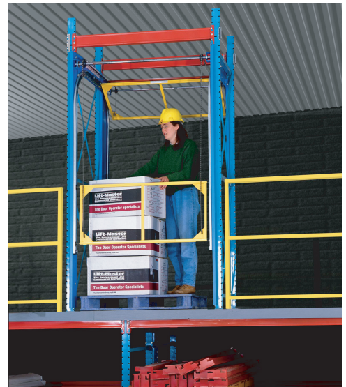
The Rack-Supported Safety Gate
