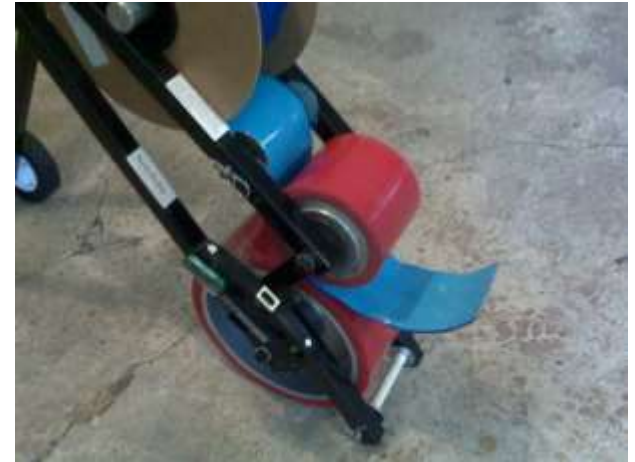
Thread Aisle Stripe Through Applicator
