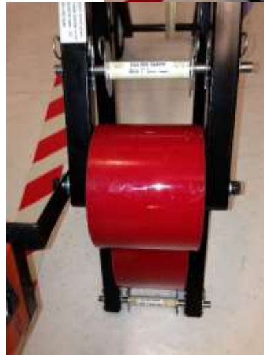
Pin and Spacer set up for 3" Wide tape
