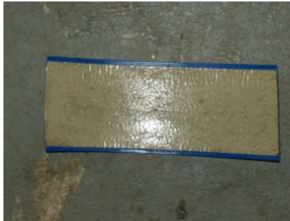
Sticky side of aisle stripe after adhering sample to a new sealed concrete floor. Floor was only swept clean. Adhesion was good but not the best. Note the contaminants on the adhesive.
