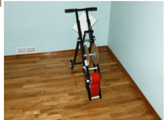
No springs or spacers are required when installing the 4" wide tapes.
