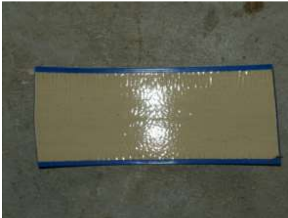
Sticky side of aisle stripe prior to adhering the sample to the floor.
