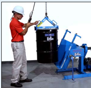
Load upright drum with crane and secure
