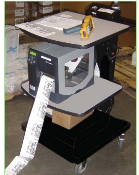
NB Series Mobile Powered Cart used in the Schwarz warehouse.
