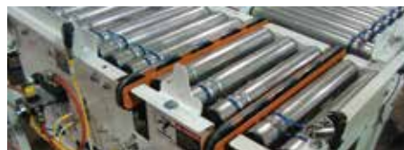
Transfer, urethane and timing belt, pneumatic and 24V actuated
