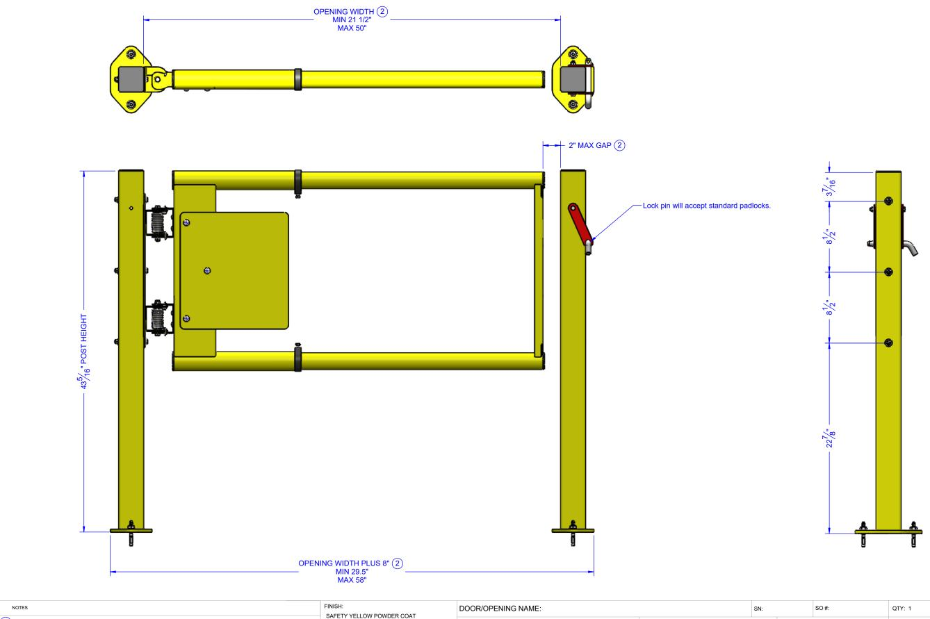
1 The gate does not contact on the free side, so there is no maximum opening width.
