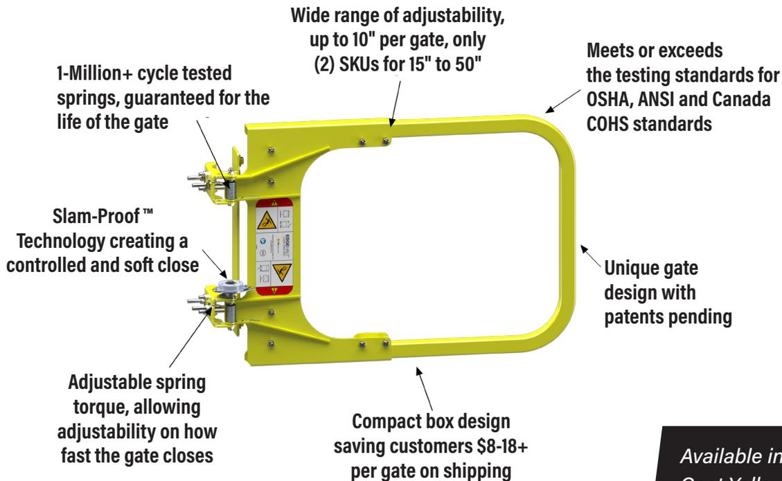
*Available in 3 Finishes - Powder Coat Yellow (PCY), Hot-Dipped Galvanized (GAL), 304 Stainless Steel Seal Welded (304SW)*
