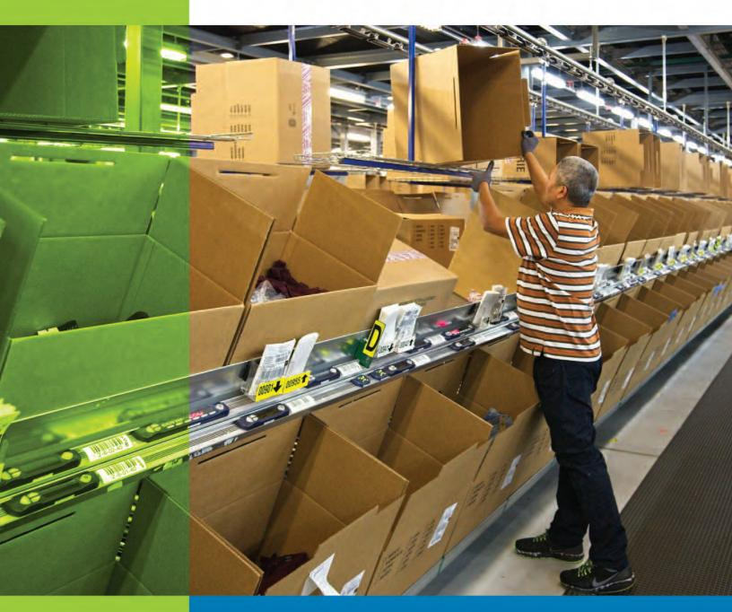
Overhead Conveyors for Distribution Warehousing
