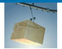
**Trash Carrier #1:** These carriers are effective for removing trash cartons from picking areas. A simple mechanical device that tips the carrier is used when the carton reaches the trash bin or trash compactor.
