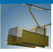
**Trash Carrier #2:** When you are generating a wide variety of trash from cartons to dunnage, a bin style carrier can be used. A simple mechanical device tips the carrier when it reaches the trash area. These can be located every 4th or 5th carrier to reduce costs.
