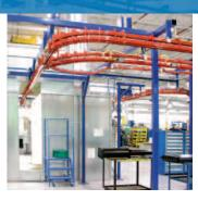
Wet spray painting of pneumatic cylinders using the **PACLINE Power and Free conveyor**.
