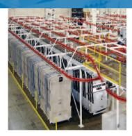
Automotive parts in a **PACLINE Power and Free live storage system** allows for unexpected production stoppages at supplier without impacting on final auto assembly plant.
