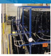
Unfinished automotive components accumulating on a multi-level **PAC-LINE™ enclosed track conveyor**.
