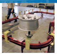
Finishing of automotive rims on rotating spindles using "slot sideways" enclosed track PAC-MAX™ conveyor.
