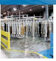
Automotive components stored in the **PAC-LINE™** automated storage and retrieval system facilitates batch building, retrieve to broadcast.
