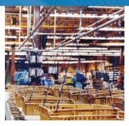
Small motor components transported in suspended baskets or totes on the PAC-LINE™ overhead conveyor.
