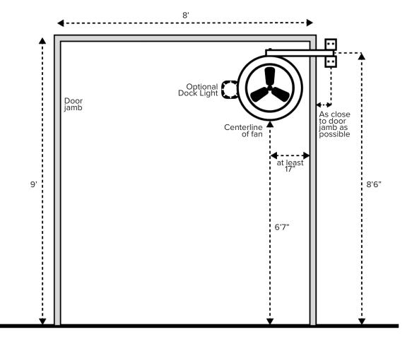
**Note:** The TC-18 is designed to purge a trailer of hot air. Mounting in the top corner pushes air through the trailer and out the opposite corner of the door, as shown below, with an exit velocity of approximately 200 FPM. The fan will not be as effective if positioned other than what is recommended or by directing on an individual.
