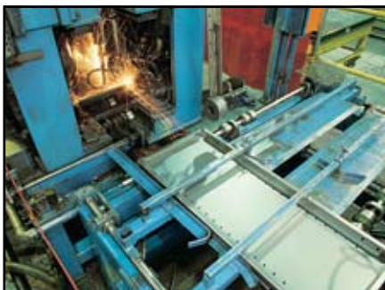
Automated welding of Hi-Performance shelves.
