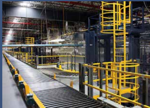
Home Appliance Lifts – M Series Mechanical VRC Ten lifts installed as a mezzanine application, including a conveyerized system. 1,200 lbs. lifting capacity; 200' per minute travel speed.
