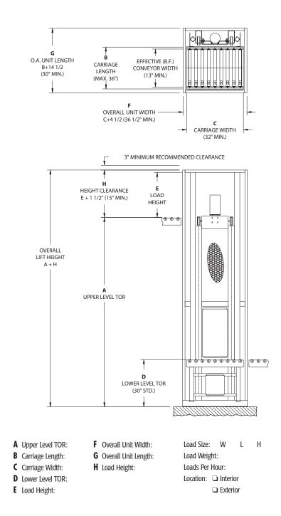
Note: The dimensions shown are illustrative. Request a job-specific drawing before making any building modifications.
