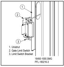
Attach Gate Limit Switch Figure 16-80
