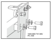
Install Interlock Keeper Assembly Figure 16-28
