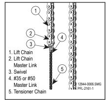
Attach the Tensioner Chain to the Lift Chain Figure 12-34
