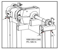
Tighten and Torque Hex Bolts Figure 12-31
