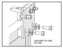
Install Interlock Keeper Assembly Figure 16-9
