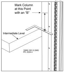
Intermediate Level Limit Switch Position Figure 14-18
