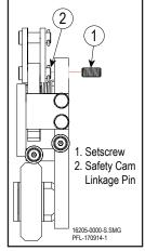
Insert Setscrew Figure 12-13 Insert Setscrew Figure 12-14
