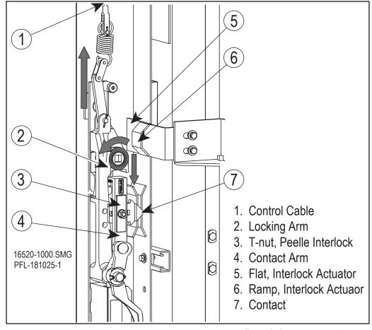
Peelle Interlock Open Position Figure 17-8
