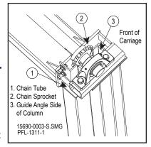
Drop the Tensioner Chain Down the Chain Tube Figure 12-35
