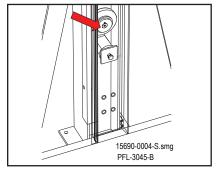
Tighten Mounting Bolt Figure 15-3
