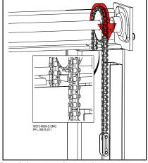
Thread Chain Over the Sprockets Figure 16-53
