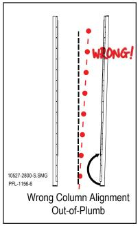
Column Alignment Out-of-Plumb Figure 12-26
