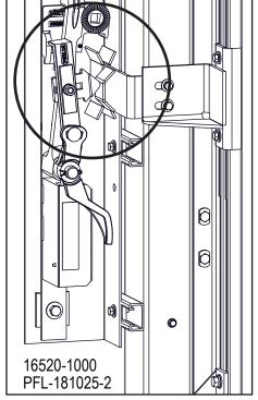
Peelle Interlock Closed Position Figure 17-9
