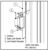
Attach Gate Limit Switch Figure 16-95
