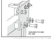
Install Interlock Keeper Assembly Figure 16-18
