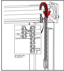
Thread Chain Over the Sprockets Figure 16-85
