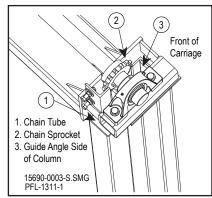
Place a Section Over the Chain Sprocket Figure 12-33
