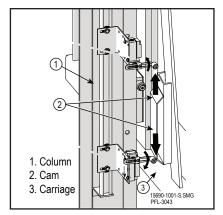
Intermediate Floor Level Limit Switch Positions Figure 14-19
