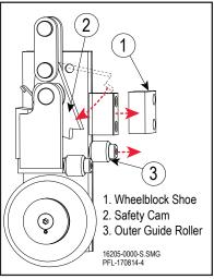
Rotate the Safety Cam Figure 12-12
