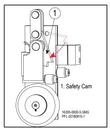
Lubricate and Rotate Safety Cam Figure 18-3
