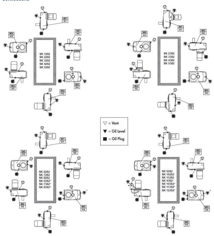
\* Oil level for 3 stage gear units
