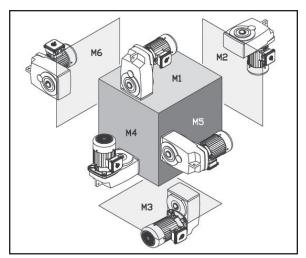
Motor and Gear Reducer Orientations Figure 11-5
