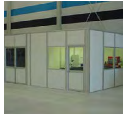
Modular walls can be designed into custom floor plans like this combination laboratory and equipment storage enclosure.
