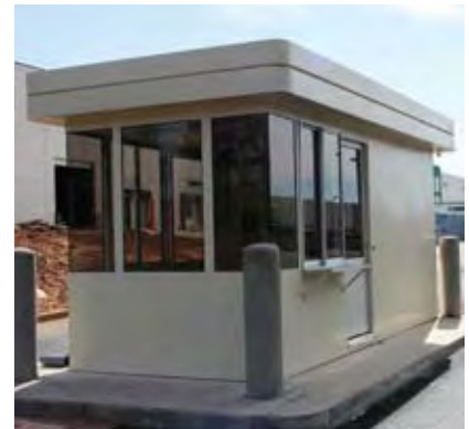
19'x8' Durasteel with tinted butt glazed, glass-to-glass corners, 18" high radius corner fascia with a 1" reveal. Included is an ADA compliant restroom.
