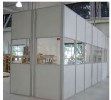
Modular walls with fixed windows quickly divide floor space to help organize plant floor operations.
