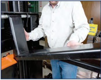
Adjustable fork carriage allows forks to be repositioned to best accommodate loads (straddle only).
