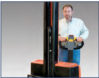
Narrow mast and offset design provide workers a clear view with no blind spots.
