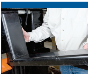
Adjustable fork carriage allows forks to be repositioned to best accommodate loads (straddle only).
