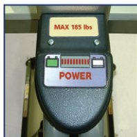
Battery indicator displays power level
