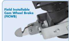
Depressing the pedal engages a non-skid pad against the wheel. Deactivate by moving the foot pedal in the opposite direction. Our field installable Cam Wheel Brakes for the 75 & 76 Series are available for roller, ball and tapered bearings on 6", 8", 10" and 12" wheels.
