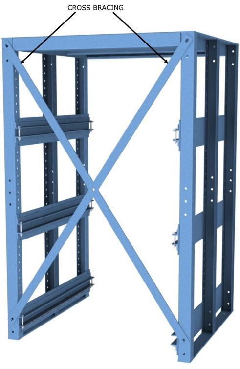
4. Level and anchor glideout frame to floor using the holes provided in the bottom pad of the uprights. Complete a final cross square check to ensure that uprights are square to each other.
