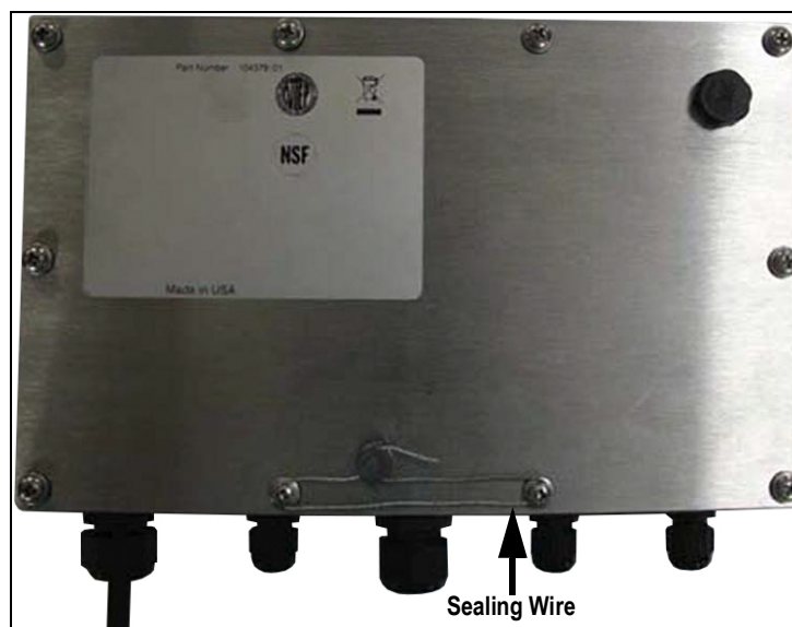
Figure 2-7. Two Point Sealing Method
