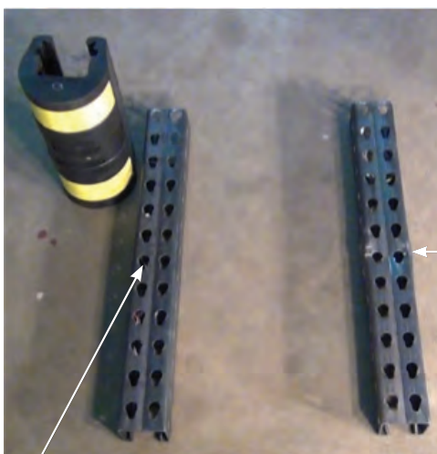
Protected 11 gage column with the RAMGuard after 20 impacts. NO DAMAGE TO EITHER COLUMN OR RAMGUARD!
