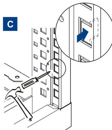
**C.** Bend tabs in cabinet front post aligned with drawer latches.
