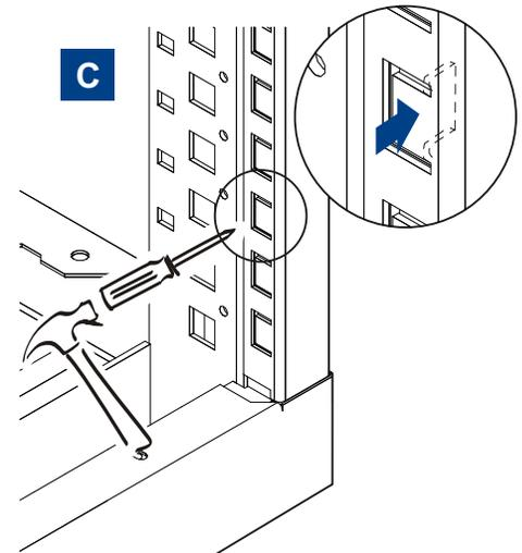
**C.** Bend tabs in cabinet front post aligned with drawer latches.
