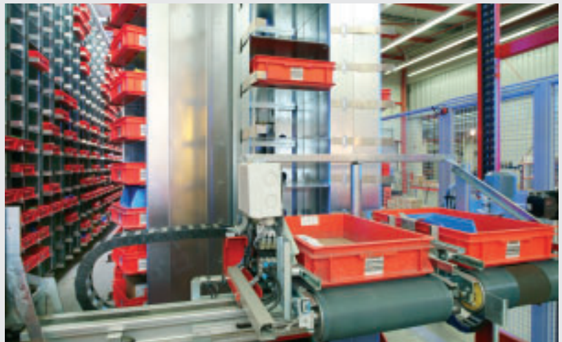
Bin retrieval and vertical transportation using stationary lifting systems. Without the use of storage and retrieval machines, small clearances between the carousels can be achieved. In this way, a lot of space can be saved.
