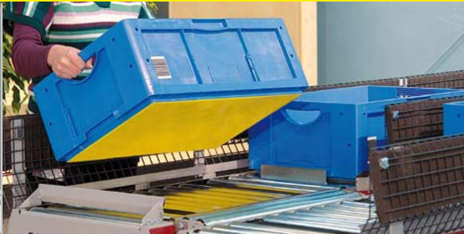
▲ Specially coated base of totes for the silent conveying system ▼ Short distances between S-Pemat and replenishment rack
