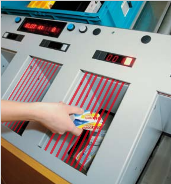
▲ Light-controlled picking guidance and hand-held terminals facilitate space to move and ensure best picking performance.
