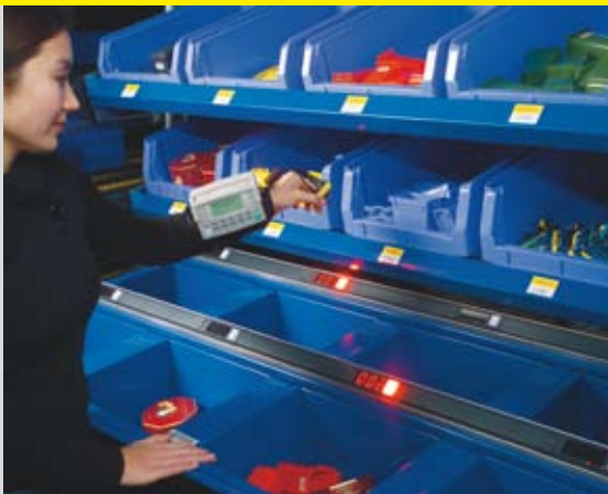
▲ Light-controlled picking guidance and hand-held terminals facilitate space to move and ensure best picking performance.
