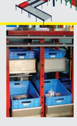
Static as well as dynamic order picking locations can be equipped, for example with Pick by Light.
