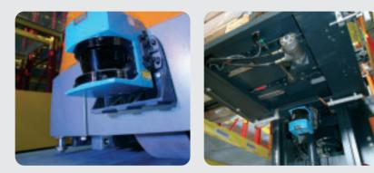
Scanning the environment, which is in real time, enables an orientation of the vehicle on the actual position of the mobile racks. Based on the same principle, the pallet shape is optically recognized during retrieval operations.
