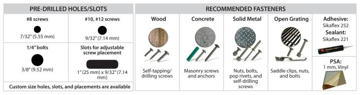
Select the appropriate fastener for the substrate to be covered. A combination of mechanical fasteners and adhesive may be used. Sikaflex 221 sealant may be used to seal edges to deter corrosion. Fasteners and pre-drilled/slotted holes are available upon request.
