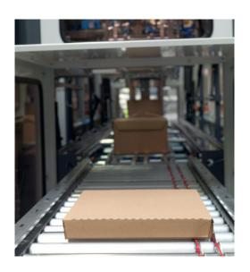
JIVARO is a parcel closing machine which adapts the height of boxes to product dimensions, in order to **reduce the size of shipments.**
