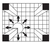
The view distance ratio is about 1 foot of viewing distance to each inch of the diameter of the dome. Due to the nature of these domes, they are made in only an 18" and 26" model.
