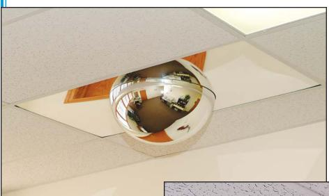
**Drop-In Domes** are easy to install into an established grid ceiling system. The 2' x 4' model is a 2-piece unit that has a full panel with a hole to match the diameter of the dome to be used. Our 2' x 2' unit is a formed one-piece dome that easily drops into a 2' x 2' grid opening.
