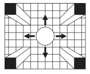
Four way intersections are the most common application for the domes. The ratio of viewing distance is estimated at one foot of viewing distance for each inch of dome diameter. In a warehouse setting, a wider viewing distance would help provide a safer view due to increased vehicle speed. The dome should be suspended as low as possible, yet taking into consideration elevated material activity.
