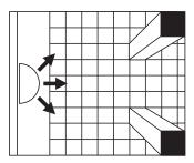
For industrial use larger domes can be mounted on the end of aisles at a lower level than most full domes. These half domes would be mounted at the end of an aisle where a forklift operator can see in both directions without needing to look towards the ceiling.
