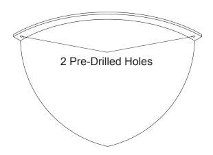
90 Degree Domes may be mounted to the ceiling by screws driven into pre-placed wall anchors.
