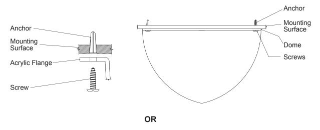
They can also be mounted by pre-drilling holes in the mounting surface and inserting a toggle bolt assembly (not included) through the pre-drilled holes on the mounting surface, then drawing the dome up by screwing the toggle bolt in.
