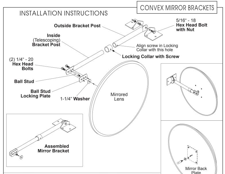
Mirror Back shows Ball Stud and Washer installing into hole in Heavy Metal Plate under back plate. Note: The Heavy Metal Plate can not be seen through back plate.
