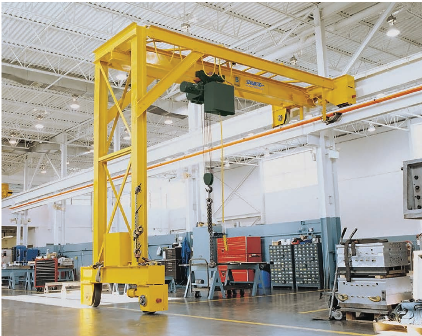
Motorized 5-ton Wide-Flange Single-Leg Gantry Crane
