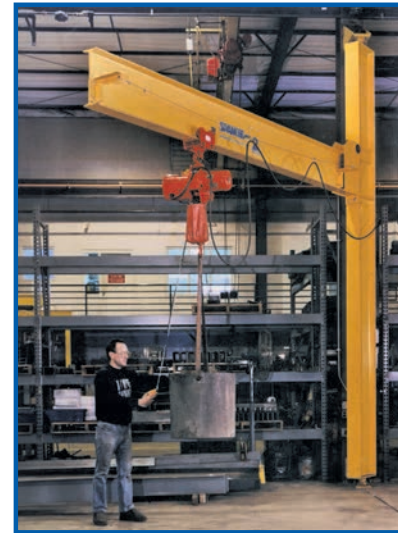
Spanco 201 Series Mast-Style Drop-Cantilever Jib Cranes are similar to the 200 Series Full-Cantilever Jib Cranes, with the addition of side-plate connections to permanently "drop mount" the boom at a specified height on the mast. This allows for clearance from overhead obstructions located below the top of the mast.
