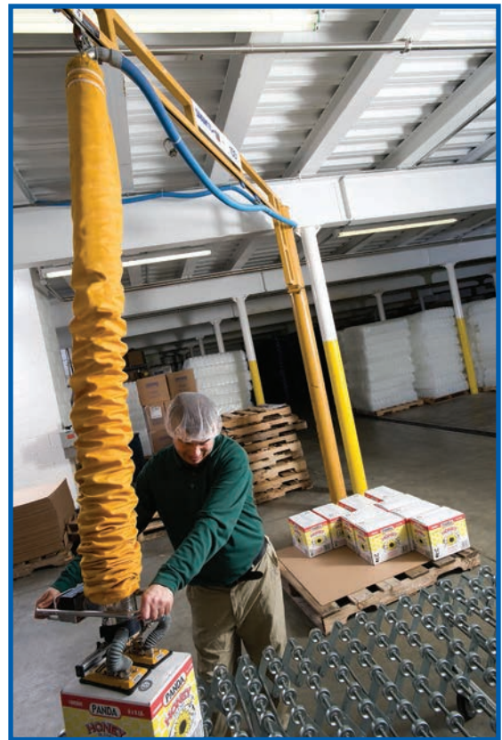
A worker stacks boxes of packaged food onto a pallet using a 150-pound capacity Spanco Freestanding Workstation Jib Crane with a vacuum attachment.
