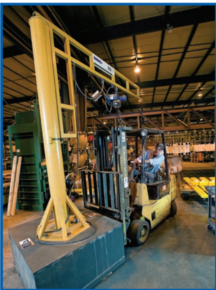
Freestanding Workstation Jib Crane with Portable Base
