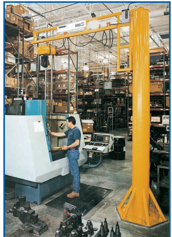
Parts are carefully lifted and positioned into this machine tool using a Spanco 500 Series Freestanding Workstation Jib Crane.
