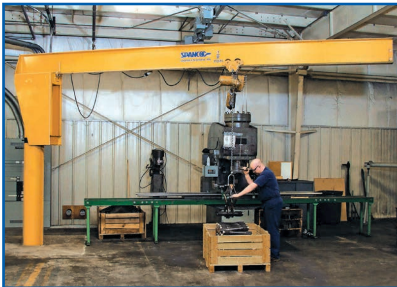
A worker lifts parts into a metalworking machine using a 1/2-Ton Spanco 101 Series Freestanding Jib Crane.
