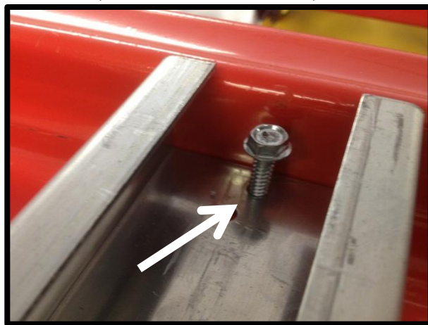
3. (Crossbar initial install detail)
