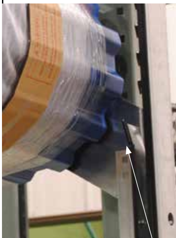
Bottom edge of guide flare aligns with bottom of notch in door mount
