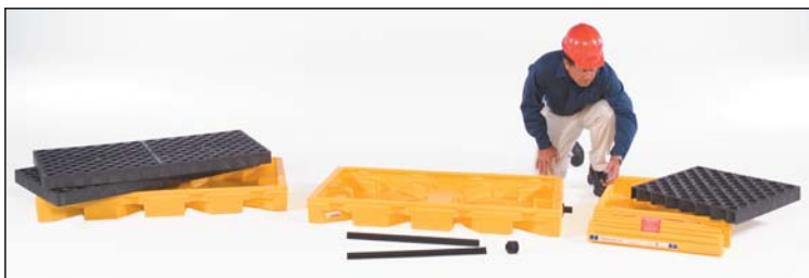
InLine Models are pre-drilled and can be quickly assembled without tools. The bulkhead fittings "lock" connected modules together and allow spills to flow from one module to the next.
