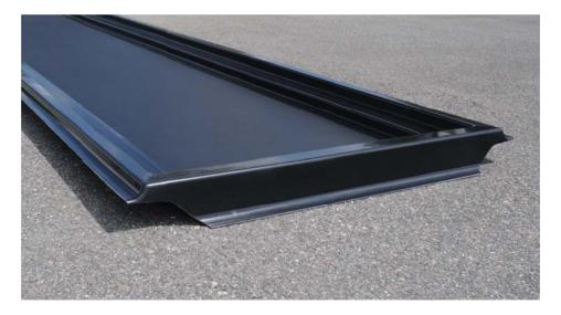
2.) It is important to install the Center Track Pans so that they are centered between the two rails. This will facilitate the installation of the Center Track Pan gaskets at the end of this process. In order to keep them centered UltraTech recommends cutting four blocks of quarterboard (5/4) wood 6 inches long. These blocks are to be used as spacers to keep the Center Track Pans centered between the two rails while assembling.
