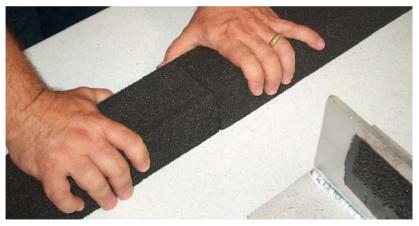
Note: the weld that has just completed will not achieve full strength for another 1 hour to 3 hours (best results are achieved if left overnight). Try not to put much stress on completed welds until they have had time to cool completely.
