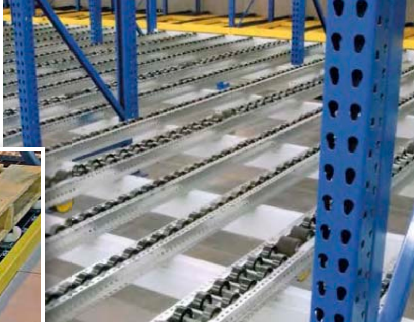
Poly-wheel deep lane pallet flow is available in single or staggered wheel configurations to fit any load. Pneumatic brakes control pallet speed
