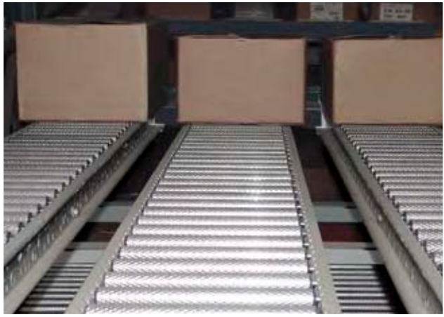
RhinoTrac lanes allow cartons to flow forward to picking position on opposite aisle with full width roller carton support.
