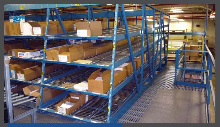
arton flow shelves full of plastic wheel rails have been the dominant solution in the light duty market for a long time. The shelves rest on pins, which install inside a steel framework, creating a carton flow system with a low initial cost but plenty of limitations.
