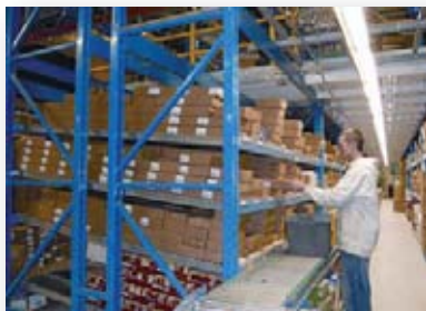
Front Pick to Gravity Push Away Combines Low Profile and High Profile Span-Track in rack and gravity pick conveyor in front.
