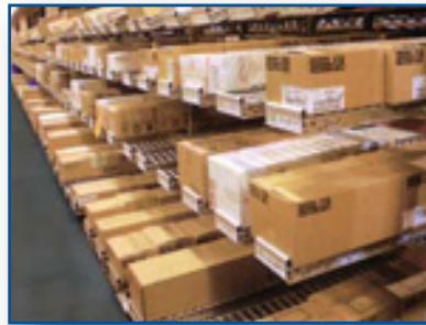
Full Case with Layback High Profile Span-Track Straight and Knuckle
