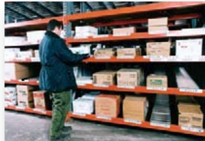
Full Case Pick / Double-Deep Roller Rack Low Profile Span-Track Throughout
