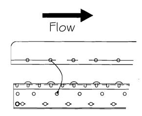
1. Center the guardrail along the edge of the track. The quardrail should be approximately the same length as the track.
