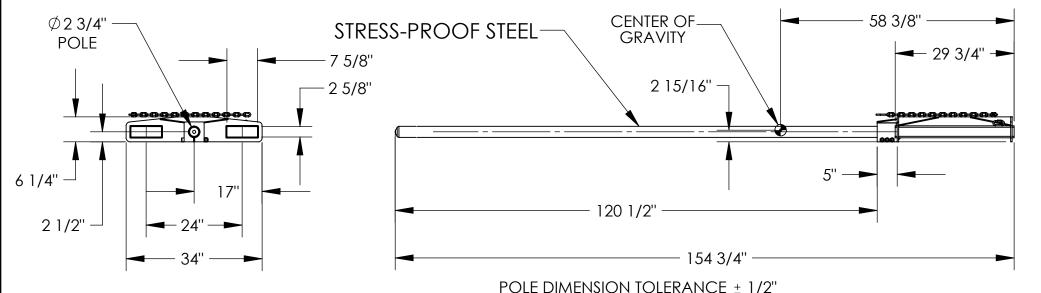
HORIZONTAL CENTER OF GRAVITY: 58 3/8" VERTICAL CENTER OF GRAVITY: 2 15/16" LOST LOAD: 380 LBS. (APPROX.)
