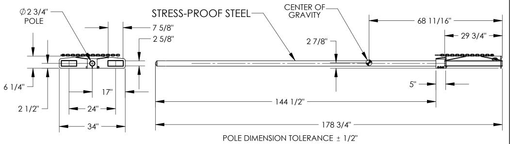
HORIZONTAL CENTER OF GRAVITY: 68 11/16" VERTICAL CENTER OF GRAVITY: 27/8" LOST LOAD: 420 LBS. (APPROX.)
