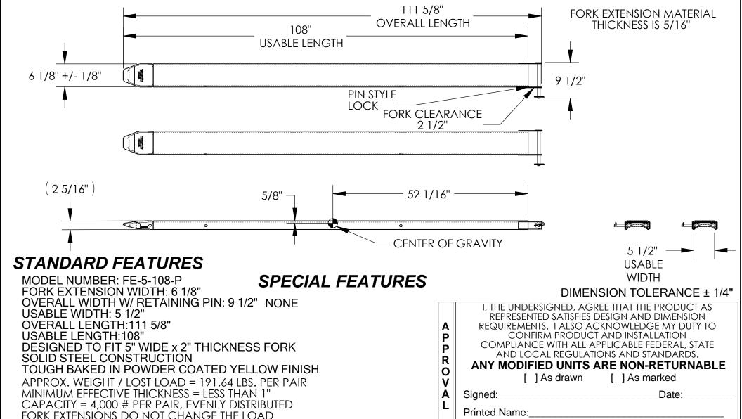
CENTER OF EXISTING FORK TRUCK. NEVER EXCEED LOAD CENTER RATING PER FORK TRUCK MANUFACTURER'S GUIDELINES. DO NOT USE THESE FORK EXTENSIONS IF LOAD WILL EXCEED FORK TRUCK MANUFACTURER'S LOAD CENTER RATING. FORK EXTENSIONS MUST NOT EXCEED 150% ORIGINAL FORK LENGTH
